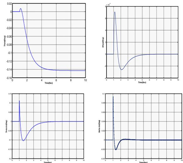
Figure 10. LQR control response of  $\alpha$ ,  $\theta$ ,  $\dot{\alpha}$  and  $\dot{\theta}$
