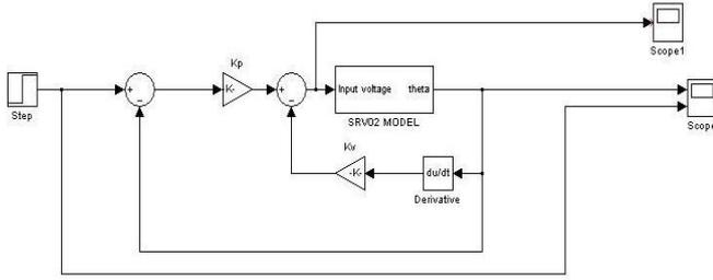
Figure 7. The position controller SRV02 model
