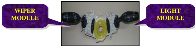
Figure 1- Schematic of a LEVER COMBINATION SWITCH
