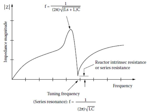
Fig[10] Resonant point on a single tuned RLC filter
