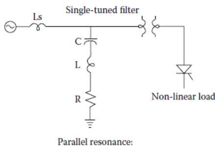
Fig[9] Single tuned filter connected system have source Load
