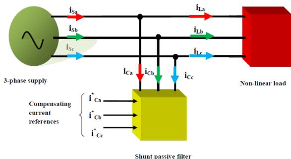
Fig[4] Schematic arrangement of passive filter connected in the system on input side
