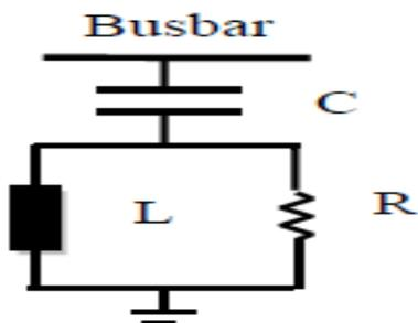
Fig[12] second order damped filter
