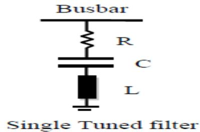
Fig[8] Simple connection diagram of single tuned filter
