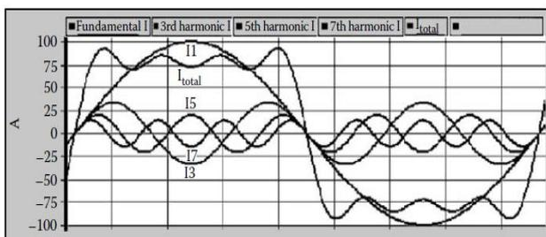
Fig [1] Resultant waveform of system has 3<sup>rd</sup> 5<sup>th</sup> & 7<sup>th</sup> harmonics
