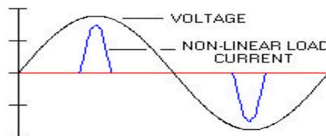
Fig [3] Waveform with Non Linear load
