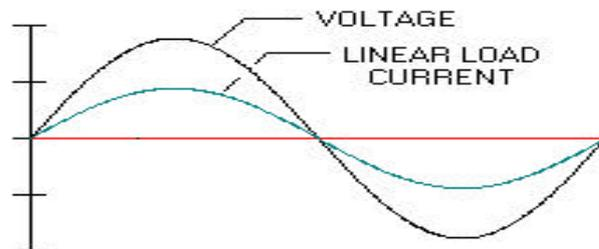
Fig[2] Waveform with Linear Load
