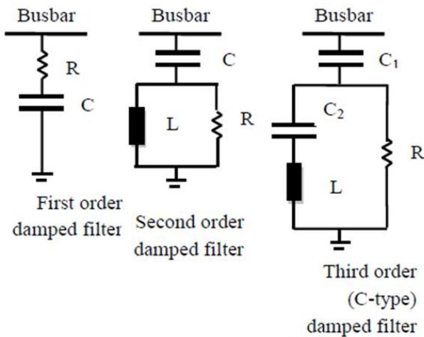
Fig[11] Different types of high pass filter arrangement
