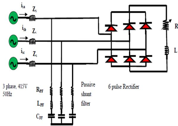
Fig[6] Shunt filter connection with six pulse rectifier circuit at input
