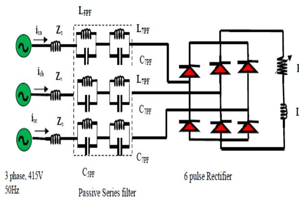
Fig 5 Schematic diagram of series connected passive filter with six pulse rectifier
