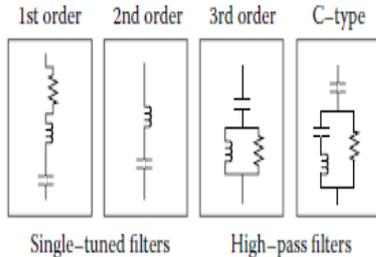
Fig[7] Different type of passive filter
