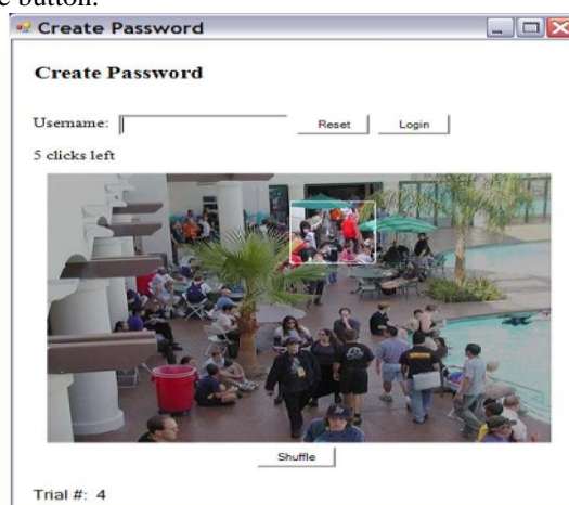
Fig. password creation in PCCP. Highlighted area is viewport (pool image is taken from [16], [1])
