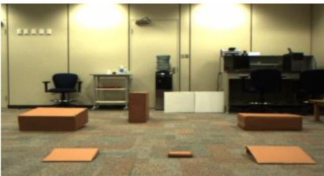
Fig. 6. The obstacle test bed consists of flat floor and objects with varying slopes and heights.
