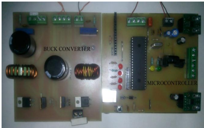
Fig. 6. Physical implementation of buck converter with microcontroller
