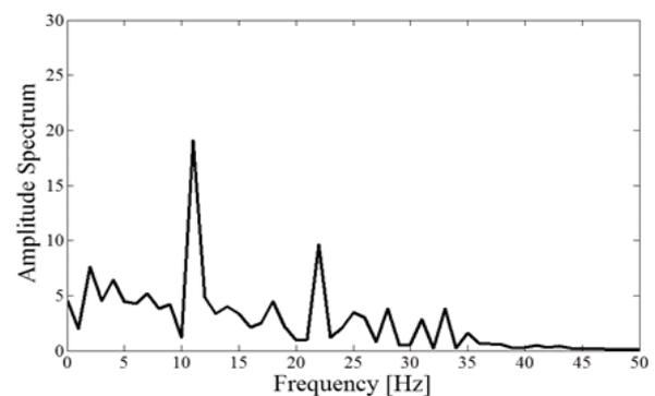
**Fig.3. Amplitude spectra of SSVEP in response to 11 Hz, recorded from Oz -A2 channel of subject 4. First and second harmonics can be found clearly.**
