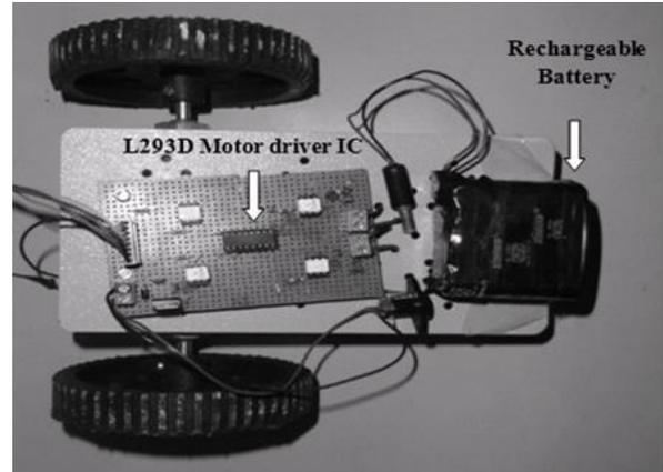
Fig.4. Wheelchair prototype for SSVEP based BCI control
