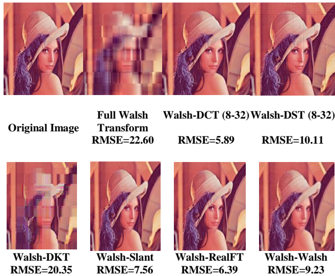
Fig. 12. Reconstructed Images at compression ratio 32 for full Walsh transform and different hybrid wavelet transforms along with their RMSE values
