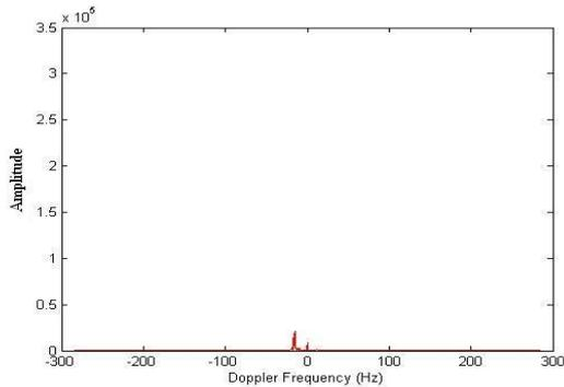
Fig 4: Signal after clutter removal
