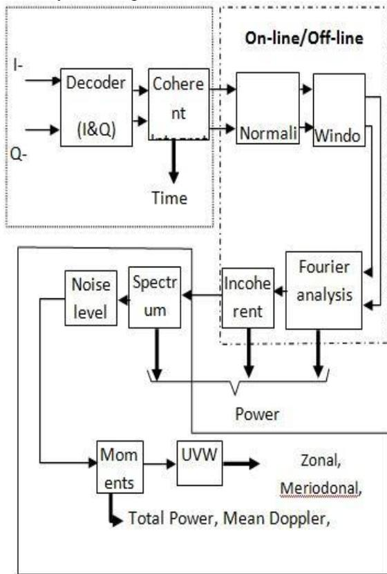
**Fig 1: Data Processing Steps of Radar Wind Profiler**
