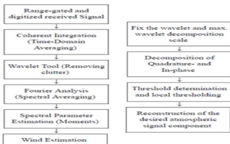
Fig 2: Left: The flow diagram using wavelet tool. Right: The wavelet algorithm flow diagram.
