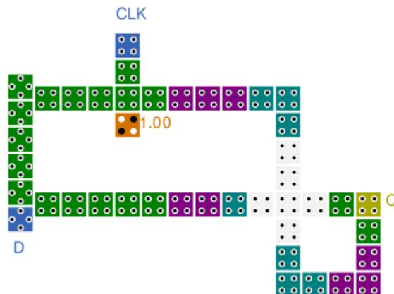
Figure 7 D-Flip-Flop
