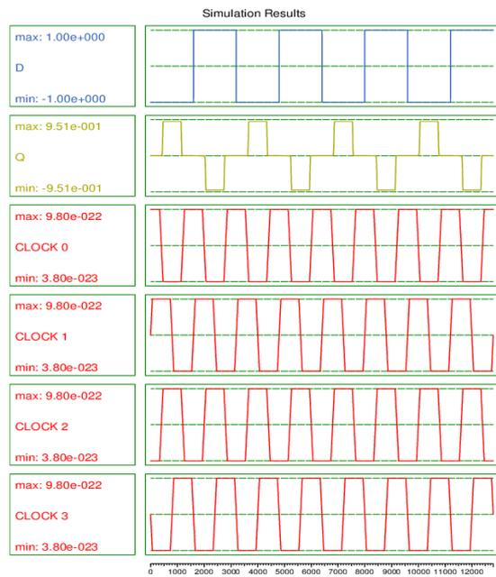
Figure 8 D-Latch (Cell-Cell Response for  $Q=1$ )
