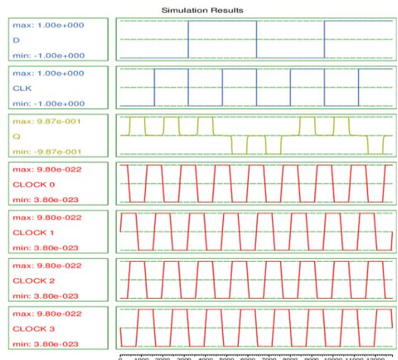
Figure 10 D Flip-Flop (Cell-Cell Response for  $Q=1$ )
