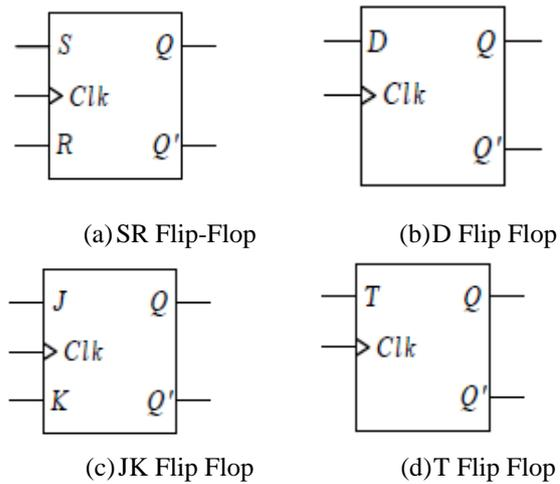
Figure 4 Four main types of Flip Flops
