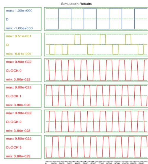
Figure 9 D-Latch (Cell-Cell Response for  $Q=0$ )
