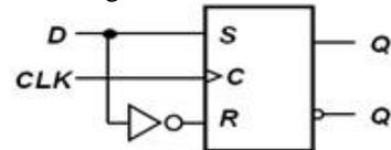
Figure 5 D- Flip-Flop from SR Flip-Flop
