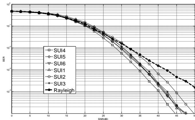
Figure 4. CPM with SC-FDE Performance Simulation
