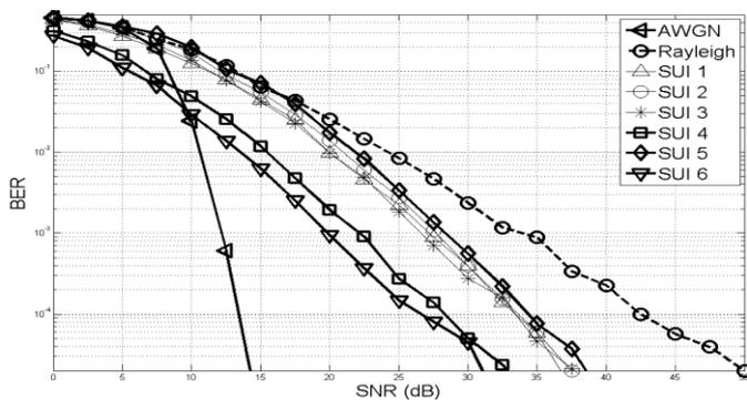
Figure 3. MCM and CPM combination Performance in SUI Channels
