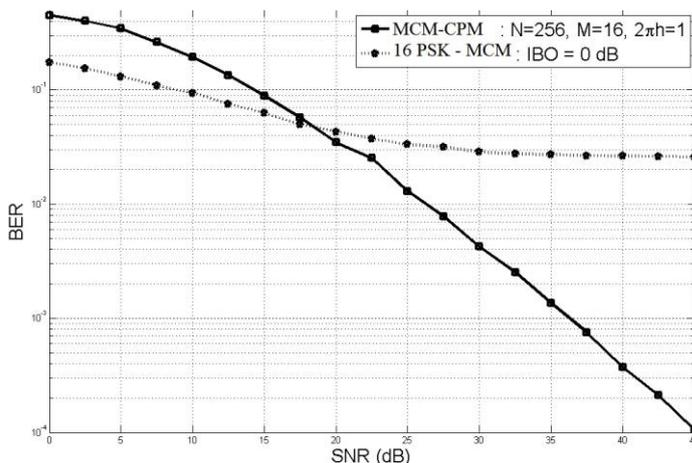
Figure 6. Performance Simulation (MCM-CPM combination and 16PSK-MCM)
