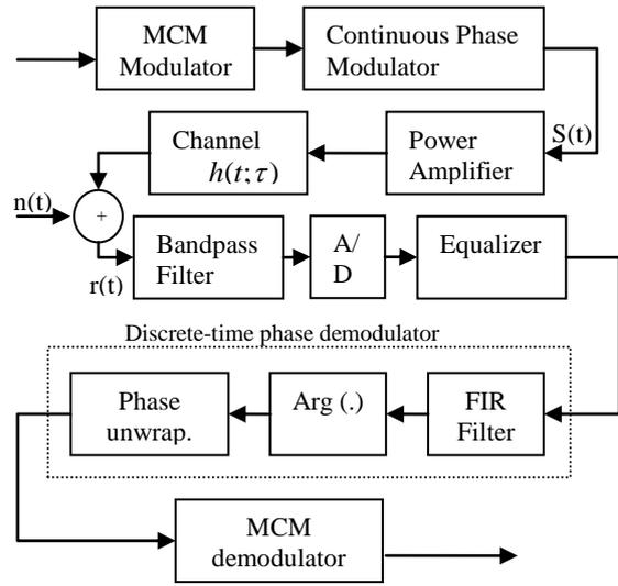
Figure 1. MCM-CPM Combination block diagram
