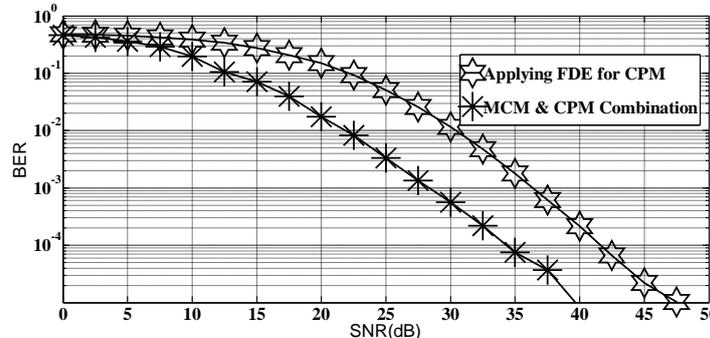
Figure 7. MCM-CPM combination and applying SC-FDE for CPM BER Performance comparison over SUI3
