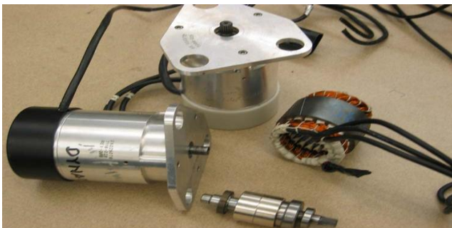
Figure 4: BLDC motor including stator and rotor.
