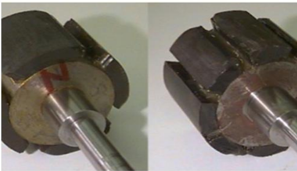
Figure 3: 4-pole and 8-pole PMBLDCM.
