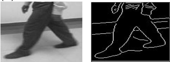
Figure. 2: image of a walking person. RGB to Grayscale (left),Edge Detected Image (right)
