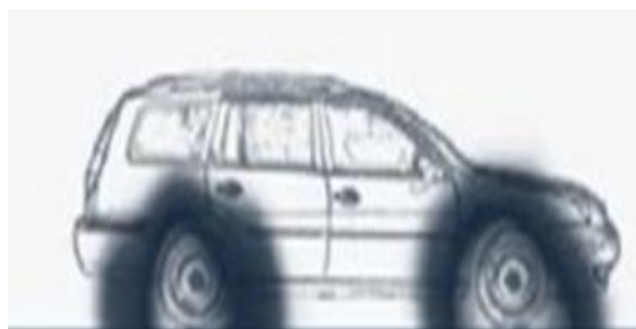
Fig .5(a) . Propagation of tyre noise of an automobile at frequency of 600 Hz
