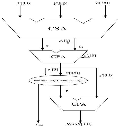
Fig. 4: One-digit, 3-operand nonspeculative adder proposed in [6].
