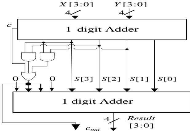
Fig. 1: Conventional hardware for performing one-digit BCD addition [26].
