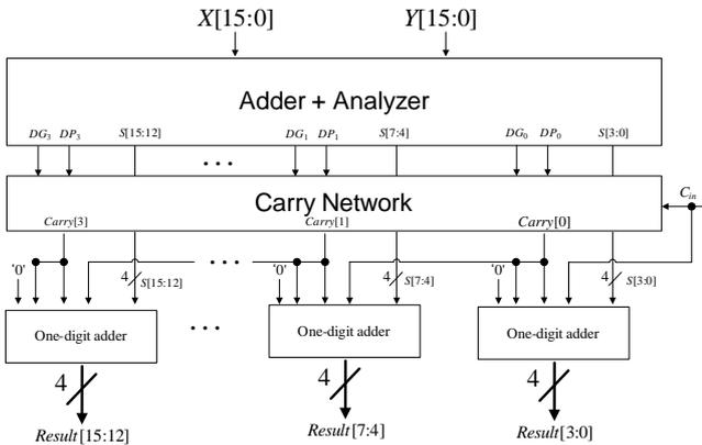
Fig. 2: The architecture of the reduced delay BCD adder proposed in [9].
