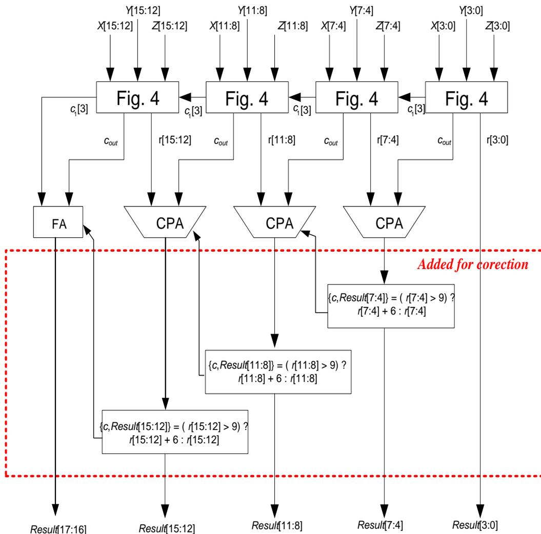
Fig. 6: The corrected architecture in [6] for nonspeculative decimal addition with three 4-digit operands.
