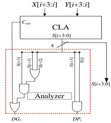
Fig. 3: The hardware of Adder+Analyzer for producing  $DG_i$  and  $DP_i$  proposed in [9].
