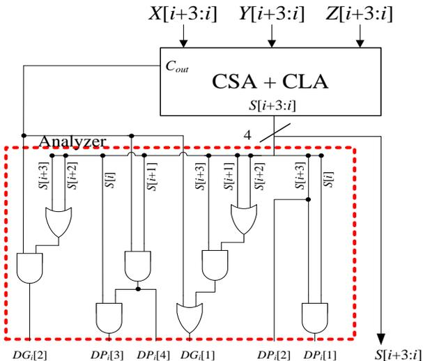
Fig. 8: One-digit hardware of our proposed CSA+CLA+Analyzer circuit.
