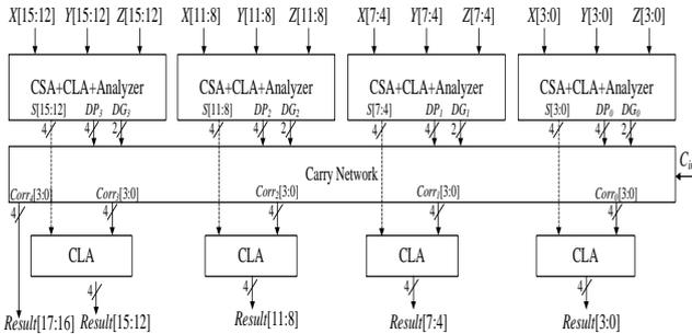
Fig. 7: The architecture of our proposed decimal adder with three 4-digit operands.
