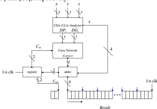
Fig 10: The architecture of our proposed digit-serial 3-operand,  $n$ -digit decimal adder.
