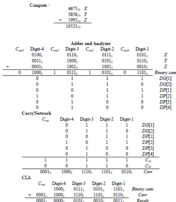
Fig. 9: Numerical example of our proposed methods.
