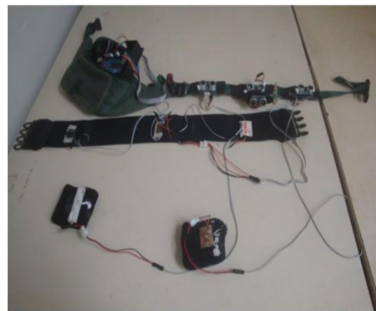
Fig. 6. Left - Vibration devices and the wearable belt, Right Coin vibration motor
