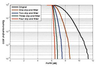
Figure 4. Comparisons of CCDF based on different iteration Clip and Filter techniques
