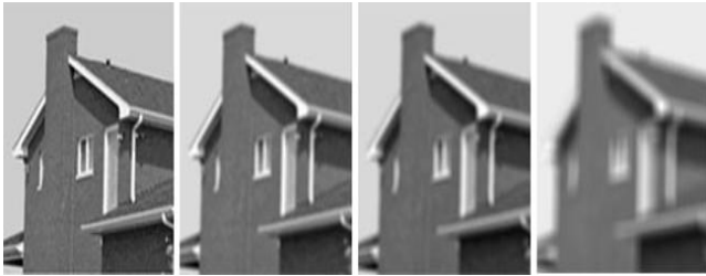
Figure 1. The Produced Scale Space by Gaussian Filter
