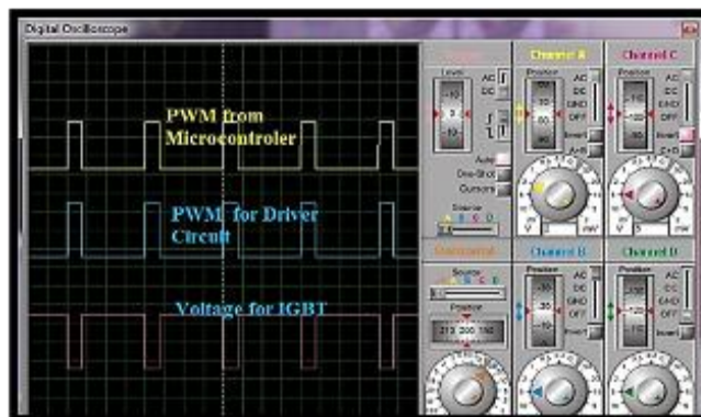
Figure 6-b: The Voltage Change on IGBT Terminals
