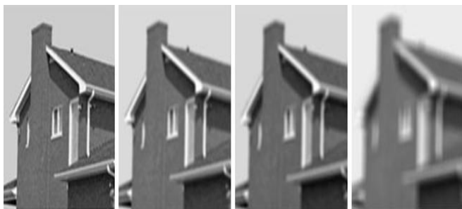
Figure 1. The Effect of Increasing \sigma of the Gaussian Function on the Image
