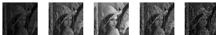
Figure 6. a) Noisy image with 0% Salt, 70% Pepper Noise & PSNR of 7.20. Restrastion results obtained for b) 'X1' with PSNR of 10.95 c) 'X2' with PSNR of 13.24 d) 'X3' with PSNR of 11.25 e) 'X4' with PSNR of 10.02.
