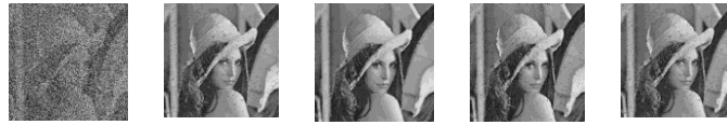
Figure 8. a) Noisy image with 30% Salt, 40% Pepper Noise & PSNR of 7.02. Restoration results obtained for : b)'X1' with PSNR of 20.47 c)'X2' with PSNR of 25.74 d)'X3' with PSNR of 23.99 e)'X4' with PSNR of 22.0
