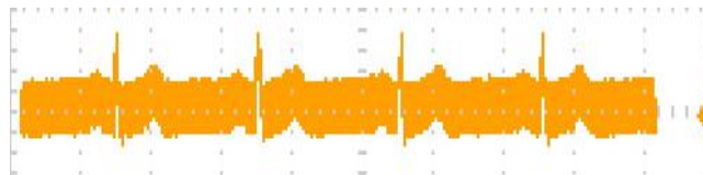
Figure 14. The simulated ECG signal of lead II with 50Hz power line noise added.
