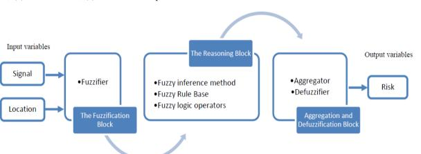
Figure 2: Structure of Fuzzy Inference System (FIS)
