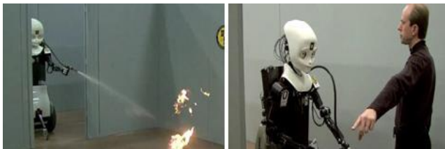
Figure 7. Octavia the fire-fighting robot of US Navy that works on Image fusion principles to understand gesture, recognize target and localize fire and extinguish it with compressed air/water supply.
