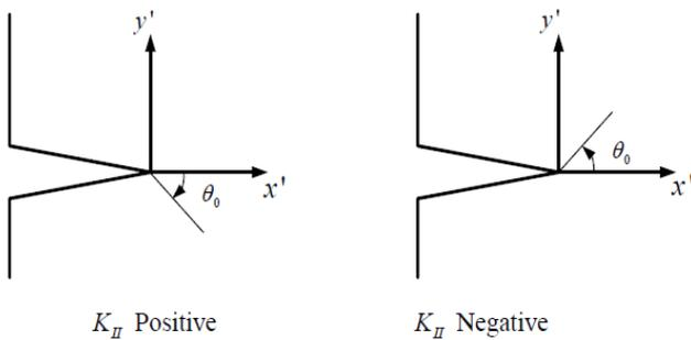
Fig. 2. Sign of the propagation angle
