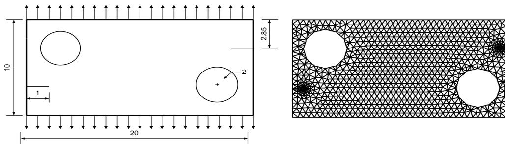
Fig. 7. Problem statement and the final mesh of the initial crack for the double edge cracked plate with two holes
