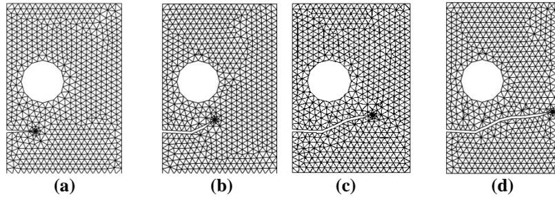
Fig. 5. Crack Growth Trajectory for Single Edge Cracked Plate with One Hole
