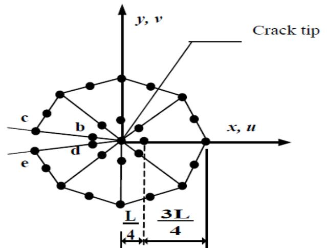
Fig. 1. Quarter-point triangular elements around the crack tip
