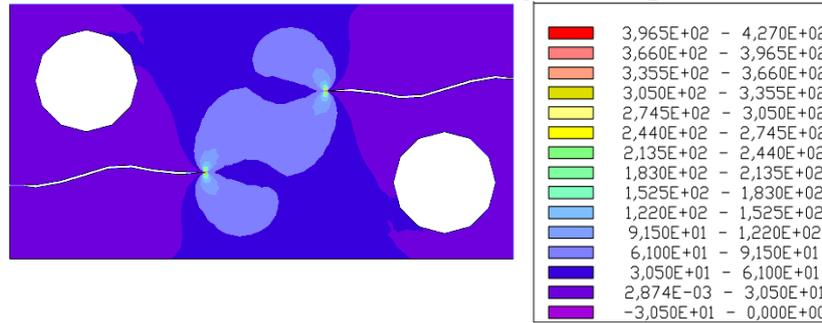
Fig. 9. Von Mises Stress field distribution at 8th step of crack propagation
