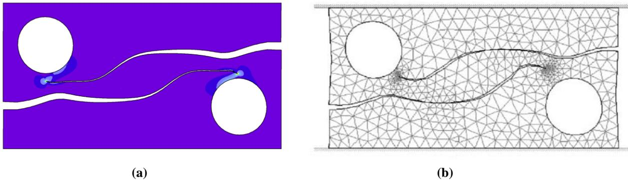
Fig. 11. Crack propagation simulation for the double edge cracked with two holes specimen (a) present and (b) Bouchard *et al.* [11].
