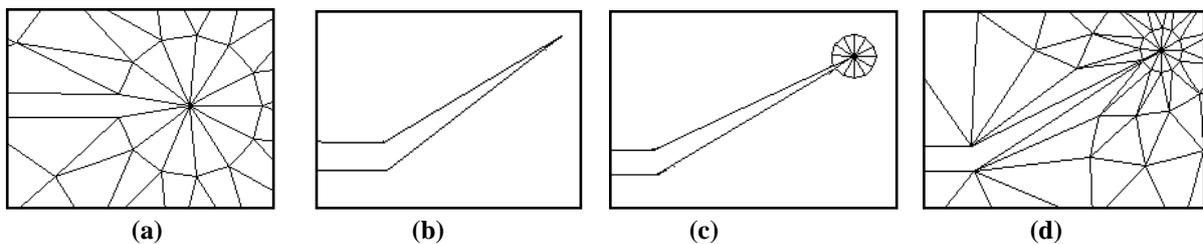
Fig. 3. Sequential procedure for geometry updating and remeshing
