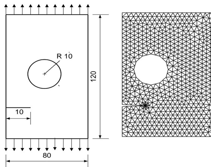
Fig. 4. Problem statement and the final mesh of the initial crack for the single edge cracked plate with one hole
