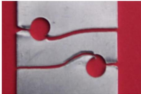
Fig. 10 Experimental cracks propagation trajectories
