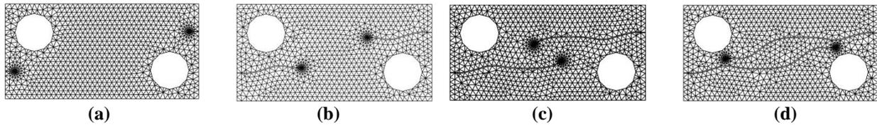
Fig. 8. Crack growth trajectory for the double edge cracked plate with two holes
