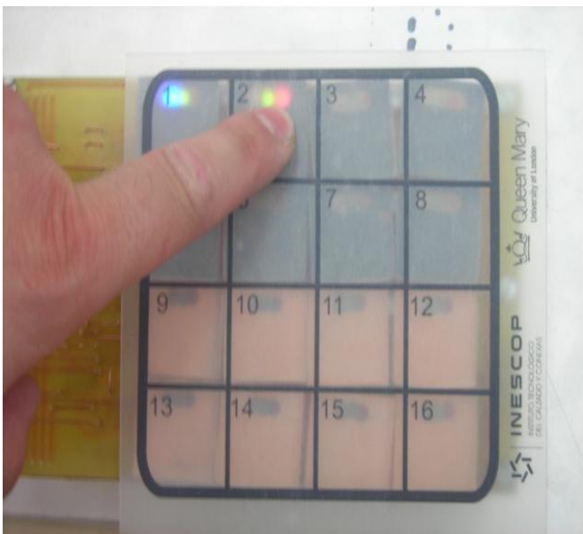
Figure 2. Portable mini-device for Stroop test software (LED design).
