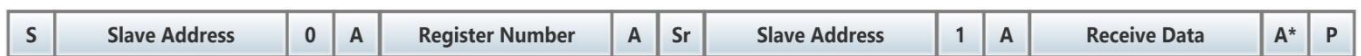
S - START condition , Sr - Repeated START condition , A - acknowledge , A* - not acknowledge , P - STOP condition ,
