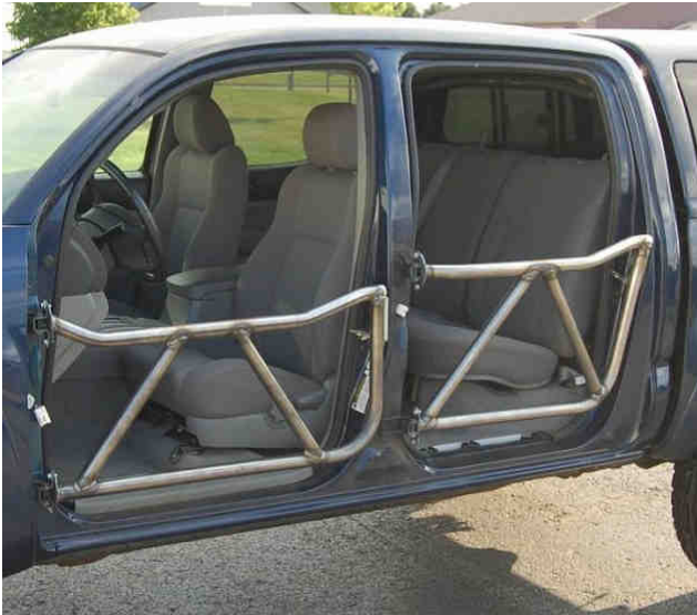
Figure 2. Tubular shape application in automotive body
