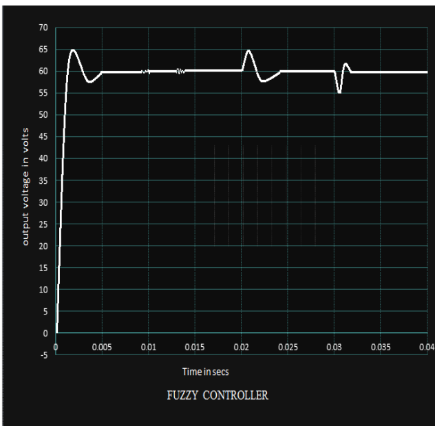
Fig. 8 Closed loop response of Triple-Lift Luo converter with fuzzy logic-controller under sudden disturbances of \pm 25\% of rated supply voltage at 0.02 sec and 0.03 sec
