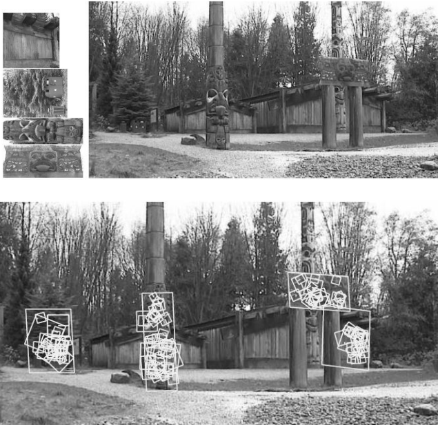
Figure 4: This example shows location recognition within a complex scene. The training images for locations are shown at the upper left and the 640x315 pixel test image taken from a different viewpoint is on the upper right. The recognized regions are shown on the lower image, with keypoints shown as squares and an outer parallelogram showing the boundaries of the training images under the affine transform used for recognition.
