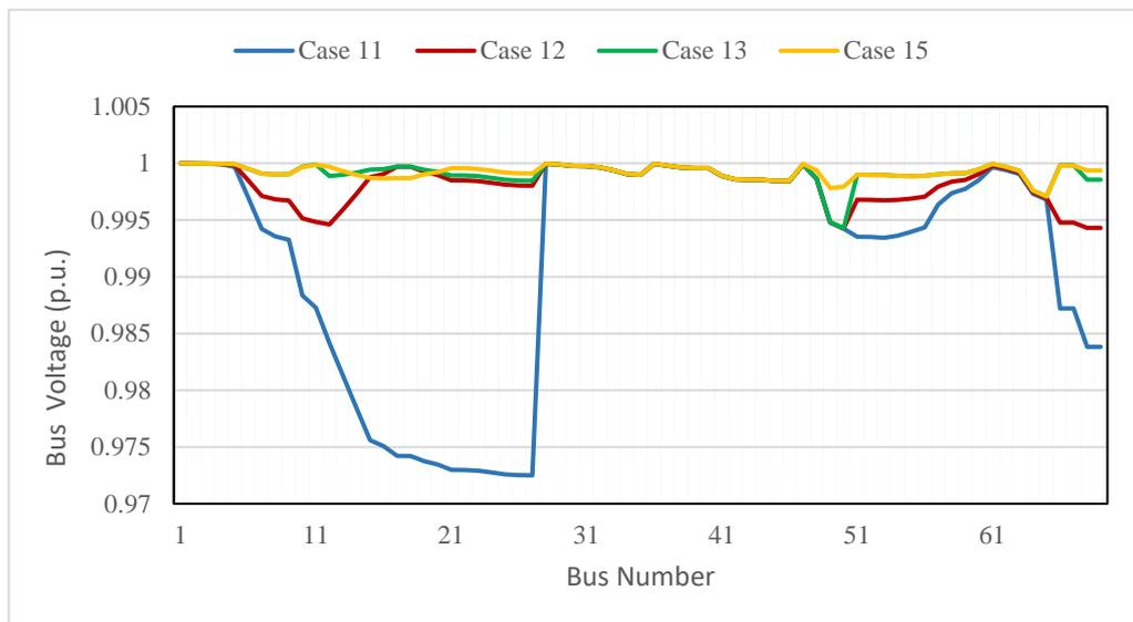
**Fig.5: Voltage profiles of buses for 69 bus system for case studies**
