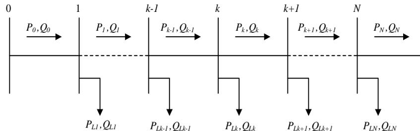
Fig.1: Single line diagram of a radial feeder
