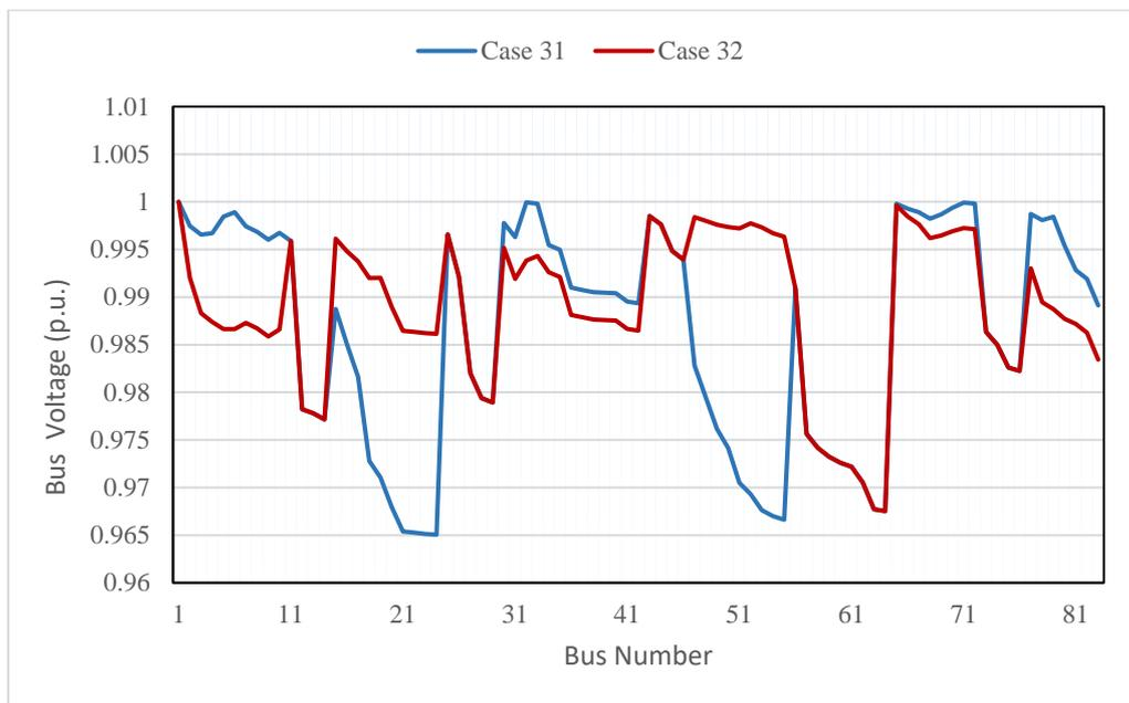
Fig.7: Voltage profiles of buses for 83 bus TPC network for case studies
