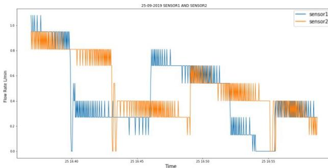
Fig. 5. Flow sensor values at different instants connected at 2 branches of the water system. (Flow rate vs Time)
