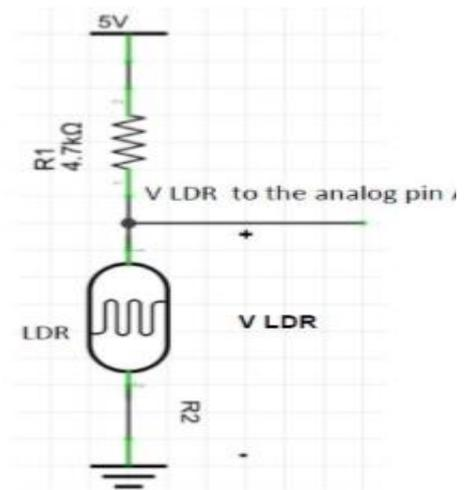
Fig. 2. Voltage divider for sensing LDR
