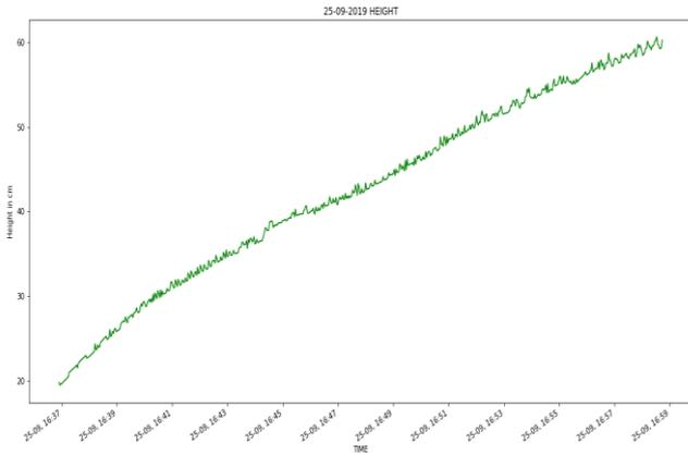
Fig. 4. Height of water in the tank vs time
